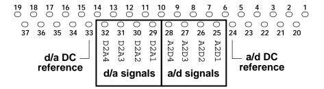
In the illustration, the a/d and d/a pins are labelled ("A2D1", "A2D2", etc.) as they are known to the BA2D and BD2A classes.
