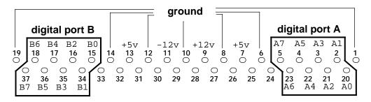
Each pin in a digital port transmits the value of a single bit; the pins are labelled by bit position. Thus, A0 is the least significant bit of digital port A, and A7 is its most significant bit. You can use any of the seven ground pins (1, 6, 8, 10, 12, 14, and 19) in your digital port circuit. The unmarked pins (24-33) are the analog ports; see "BA2D and BD2A" on page 9 for more information on these ports.
