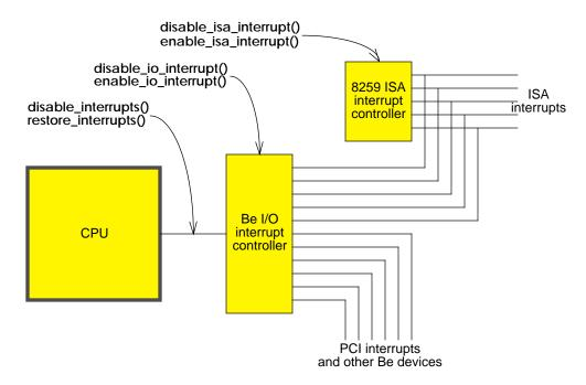
Interrupts that have been disabled by disable\_interrupts() must be reenabled by restore\_interrupts().
